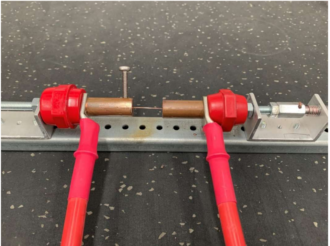
Arc test device showing a test wire ready to test.
