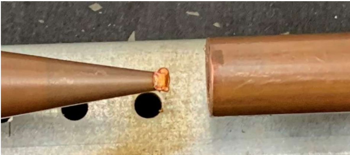
Arc Test Device showing the remains of the rod after Arc Test 6. Note the gap is 5.6mm but the burn marks are out to 7.5mm.
