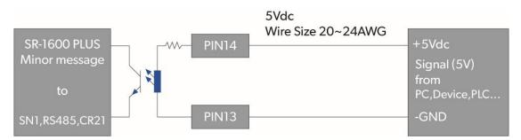
Figure 9-4. Application diagram of dry contact pin14~13(Minor)
