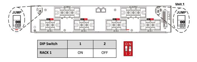
Figure 17-1. Parallel Connection via jumper setting
