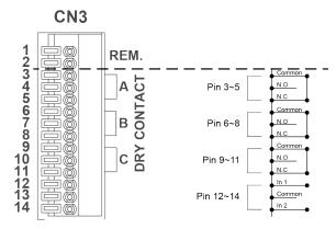
Figure 9. CN3 dry contact pin assignment
