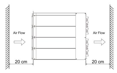
Figure 15. SR-1600 PLUS installation space requirement
