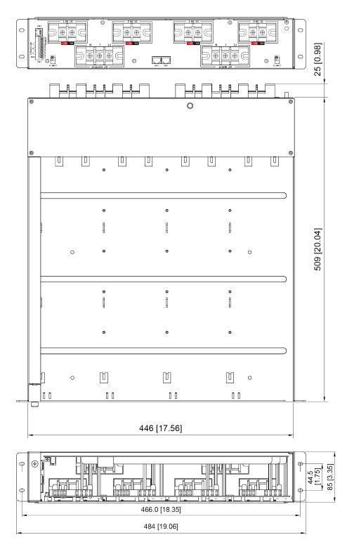
Figure 2. SR-1600 PLUS mechanical drawing-rack
