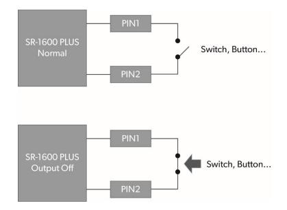
Figure 9-5. Application diagram of dry contact pin1~2
