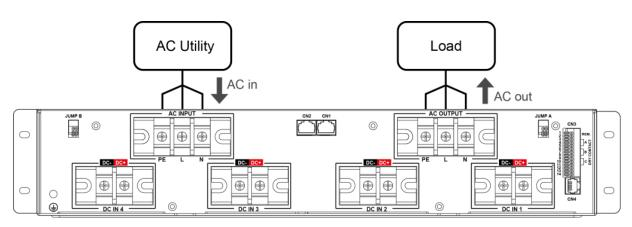
Figure 10. AC terminal connection
