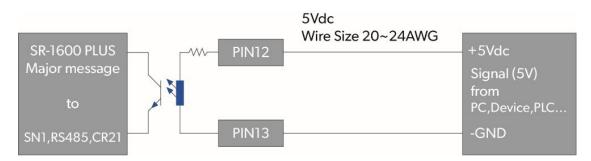
Figure 9-3. Application diagram of dry contact pin12~13(Major)
