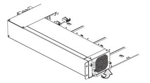
Figure 19. Remove the inverter module: step 1
