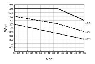
Figure 4. SR-1600 PLUS de-rating curve: SR-1600-148/248 PLUS
