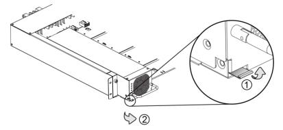
Figure 20. Remove the inverter module: step 2
