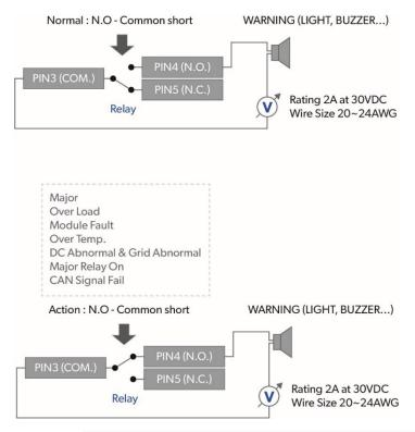
Figure 9-1. Application diagram of dry contact pin3~5(Major)
