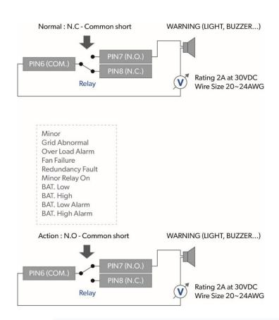
Figure 9-2. Application diagram of dry contact pin6~8(Minor)
