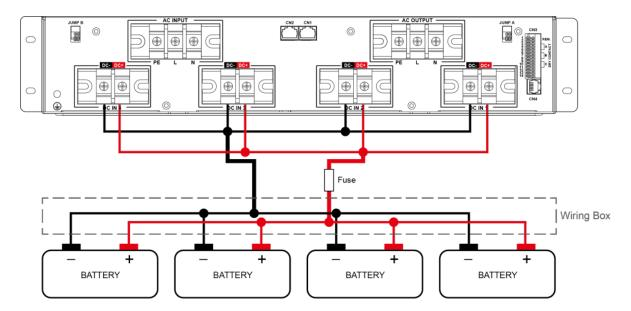
Figure 13. SR-1600 PLUS battery cabling (multi battery I)
