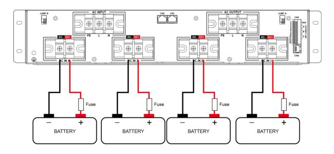
Figure 14. SR-1600 PLUS battery cabling (multi battery II)
