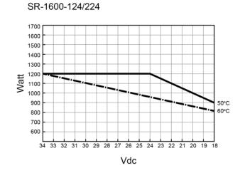
Figure 3. SR-1600 PLUS de-rating curve: SR-1600-124/224 PLUS
