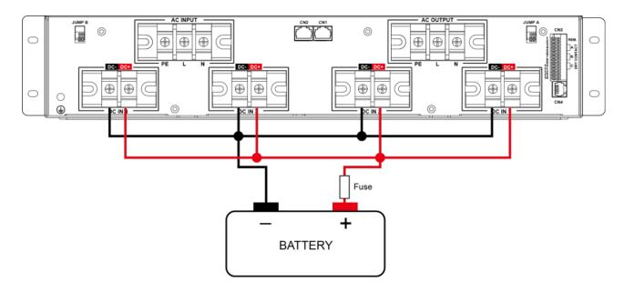
Figure 12. SR-1600 PLUS battery cabling
