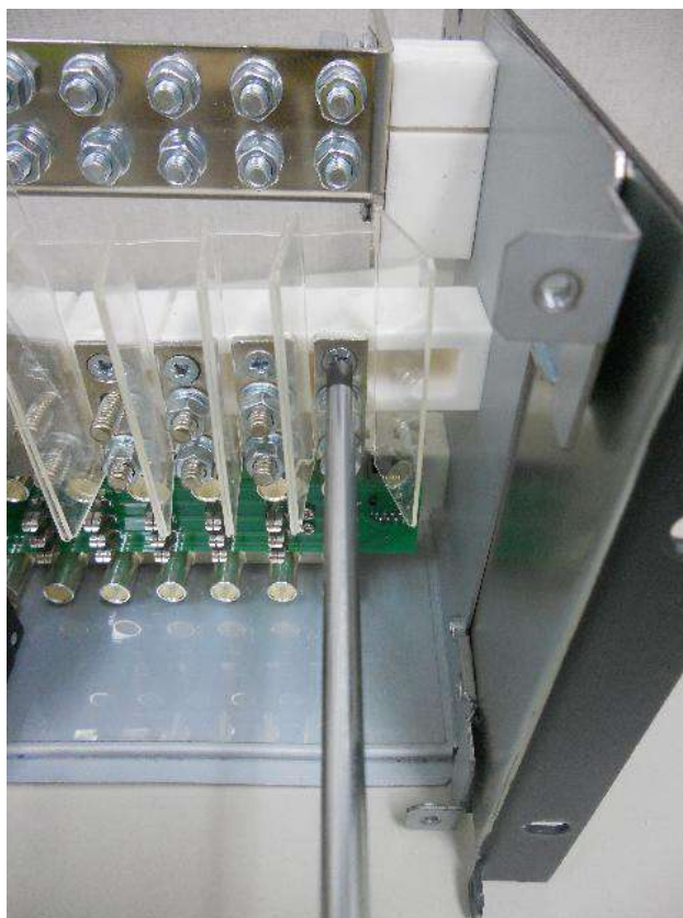
Screwdriver removing insulator fixing screw
