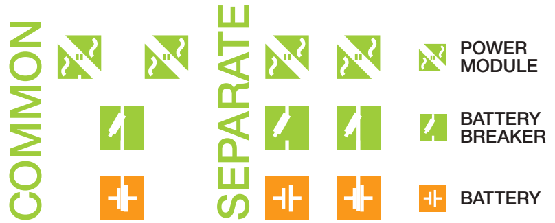
Common versus Separate Battery configuration
